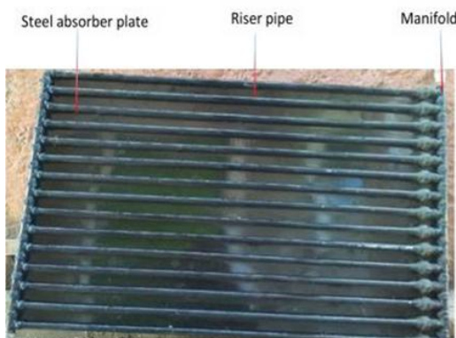
Fig. 3: Absorber plate with pipes
